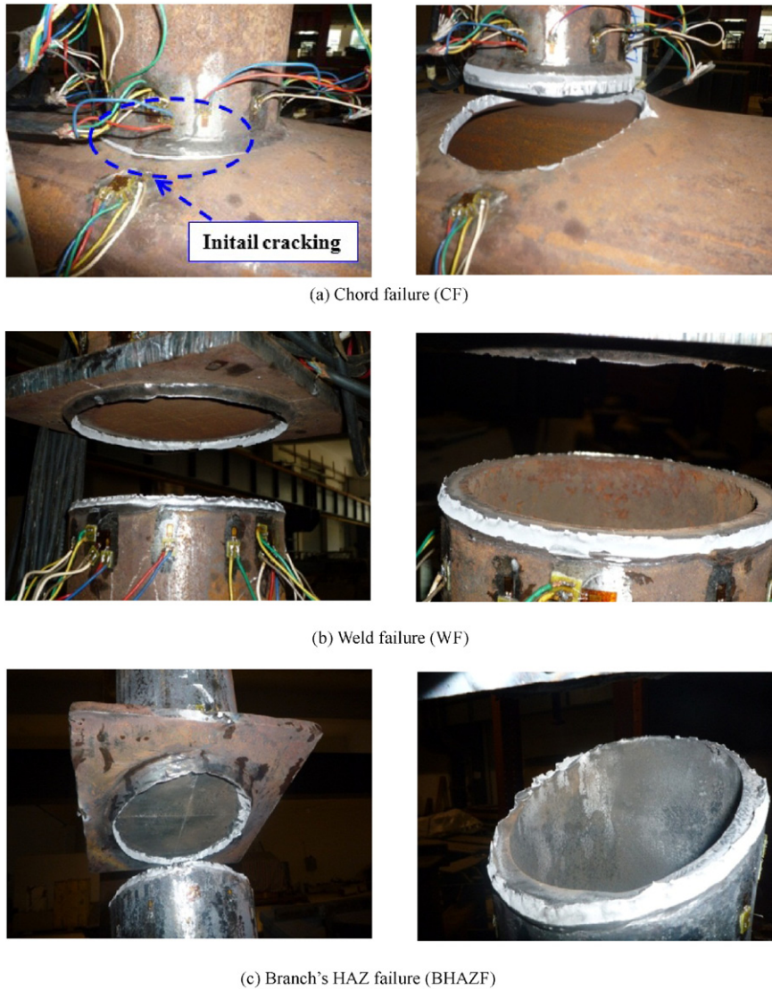
Fig. 9. Failure modes of specimens.
