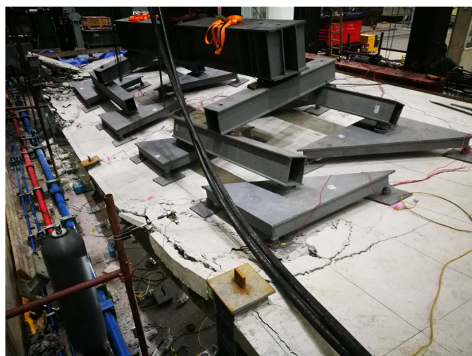
Fig. 15. Failure phenomenon at the end of the test.
